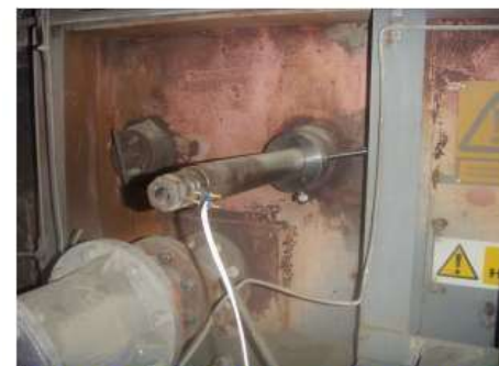
Cardox Tube inserted through Socket into snowman and secured Tube is then activated
