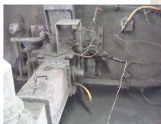
CARDOX TUBES Applied around discharge area of silo
